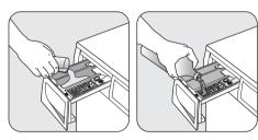
Pull out the dispenser drawer until it stops. Measure out the amount of detergent required, pour it into the main wash compartment UU or in the appropriate compartment if the selected programme/option it requires (see more details in "Detergent dispenser drawer"). If required, pour fabric softener into the compartment marked  $\mathfrak{B}$  (the amount used must not exceed the «MAX» mark in the drawer). Close the drawer gently.
